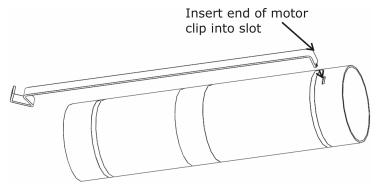
**Step 2** – While holding the motor hook in the slot, apply glue around the motor tube between the wide marks. Push the slotted motor sleeve over the motor hook until the ring is between the wide marks on the motor tube.
