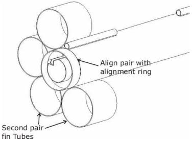
**Step 5** – Apply glue in a thin line along the length of the last fin tube pair in 2 places and the launch lug. Refer to the fin tube layout guide on previous page for glue locations between the lower body tube, fin tubes, and the launch lug. Attach the last fin tube pair to the body tube, second tube pair, and launch lug while aligning with the line around the tube as shown. Set to dry.
