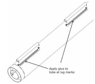
**Step 2** – After the launch lugs have dried, apply a thin layer of glue between the body tube and both launch lugs with your finger to create a fillet that will strengthen the launch lugs. Set aside to dry.
