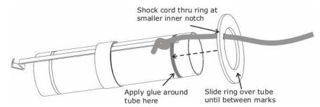
**Step 5** – Apply glue around the motor tube between the marks near the bottom of the tube. Push the centering ring with the larger slot over the motor hook until it is between the marks.
