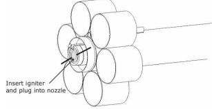
**Step 4 –** Install model rocket motor igniter according manufacturers recommended procedure.
