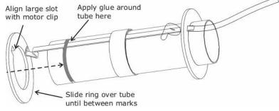
**Step 6** – Apply glue around the inside of the top end of the motor tube and push the thrust ring in until against the motor hook and flush with the end of the motor tube. Set aside to dry thoroughly.
