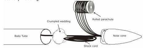
**Step 2** – Insert the folded parachute into the lower body tube, then insert the payload section to complete the recovery assembly.
