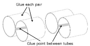
**Step 3** – Apply glue in a thin line along the length of the first fin tube pair in 2 places and the launch lug. Refer to the fin tube layout guide on this page for glue locations between the lower body tube, fin tubes, and the launch lug. Attach the first fin tube pair to lower body tube and launch lug while aligning with the line around the tube as shown.
