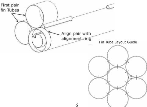
**Step 4** – Apply glue in a thin line along the length of the second fin tube pair in 3 places. Refer to the fin tube layout guide on previouse page for glue locations between the lower body tube and the fin tubes. Attach second fin tube pair to the lower body tube and first fin tube pair while aligning with the line around the tube as shown.
