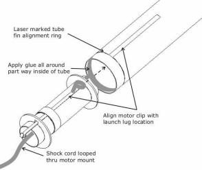
**Step 4** – Pull the shock cord back thru the body tube and out the top of the body tube. Apply a glue fillet at the centering ring and body tube attachment joint. Set aside to dry with the motor mount side of the airframe tube facing up.
