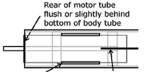
Front of ring flush or slightly behind bottom of 3 slots Motor hook between slots aligned with launch lug mark
