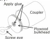
**Step 2** – Apply a thin bead of glue around the inside edge of the payload tube and insert the bulkhead assembly until it is  $\frac{1}{2}$ " from the end of the payload tube.
