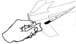
**Step 2** – Apply sanding sealer to the fins and let dry. Sand the fins with #240 grit sandpaper between coats of sanding sealer. Re-do this process until the fins are smooth and the balsa grain is filled.
