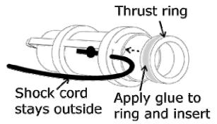
**Step 6** – Loop the yellow kevlar shock cord through the thrust ring end of the motor tube. The rings should be positioned as shown.
