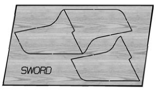
**Step 2** – Sand the leading edge and the tip of each fin round. Leave the root of the fin where it inserts and attaches to the body tube square.
