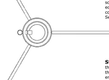
**Step 5** – After the fins and launch lug have dried, apply a thin layer of glue between the body tube and the fins, and the body tube and launch lug with your finger to create a fillet that will strengthen the fins and launch lugs. Set aside to dry. Check the fin alignment to make sure they are 120 degrees apart while drying.
