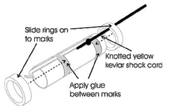
**Step 5** – Apply glue around the outside of the thrust ring and insert into the motor tube at the end where the motor hook is inserted. Push in until against the motor hook and flush with the end of the motor tube.
