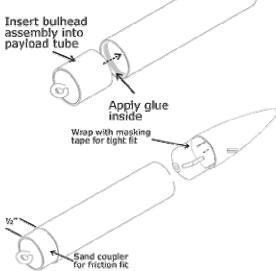
**Step 3** – Check the fit of the coupler in the body tube. If necessary, sand with #240 grit sandpaper for a friction fit (usually not necessary). Wrap masking tape around the shoulder of the nose cone for a snug fit in the payload tube.
