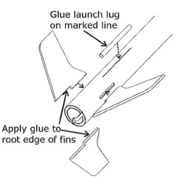
**Step 4** – Apply a thin bead of glue along the length of the launch lug and attach to the body tube where the launch lug line is marked. Allow to dry for ½ hour or more.
