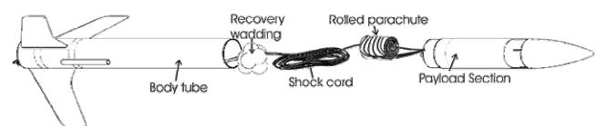
**Step 2** – Fold the parachute and roll up small enough to fit into the rocket body tube. Insert the parachute into the rocket body tube and insert the nose cone to complete the recovery assembly.
