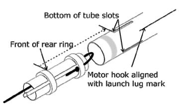
**Important:** Do the following motor mount insertion in one move. Do not stop until the motor mount is in the correct position.
