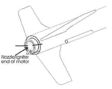
**Step 4** – Insert the rocket motor with the nozzle/igniter end facing the rear of the rocket. The motor should clip into place with the motor hook retaining the motor.
