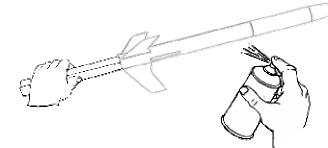
**Step 4** – Apply a first thin color coat of gloss spray enamel to the whole rocket using even back and forth movements.
