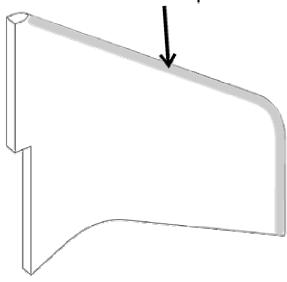
**Step 3** – Apply a bead of glue to the root edge on each fin and insert the root tab of each fin into the fin slots on the body tube. The front root edge of the fins should glue against the motor tube inside and the rear root edge against the body tube outside.
