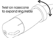
**Step 4** – While holding the motor hook in the slot, apply glue around the motor tube between the marks. Push the expanded end of the centering rings over the motor hook with the knotted end of the kevlar shock cord
