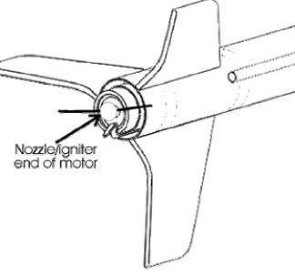
**Step 4** – Insert the rocket motor with the nozzle/igniter end facing the rear of the rocket. The motor should clip into place with the motor hook retaining the motor.
