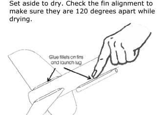
Step 5 - After the fins and launch lug have dried, apply a thin layer of glue between the
