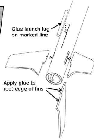
**Step 4** –Apply a thin bead of glue along the length of the launch lug and attach to the body tube where the launch lug line is marked. Allow to dry for ½ hour or more.
