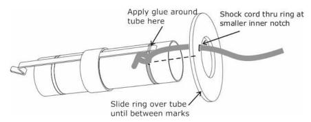
**Step 5** – Apply glue around the motor tube between the marks near the bottom of the tube. Push the centering ring with the larger slot over the motor hook until it is between the marks.
