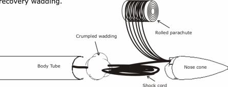
**Step 2** – Insert the folded parachute into the lower body tube, then insert the payload section to complete the recovery assembly.
