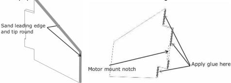
**Step 2** – Apply glue to the root edge and tab of each fin and place each fin into the fin slots near the bottom of the body tube. The fins should be against the motor tube between the centering rings with the fin motor mount notch over the motor clip sleeve.
