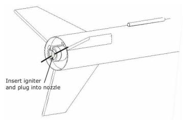
**Step 4** – Install model rocket motor igniter according manufacturers recommended procedure.
