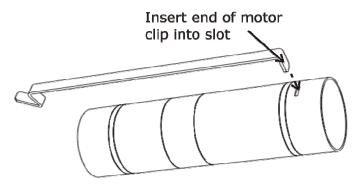
**Step 2** — While holding the motor hook in the slot, apply glue around the motor tube between the wide marks. Push the slotted motor sleeve over the motor hook until the ring is between the wide marks on the motor tube.
