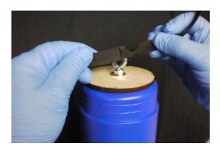
Step 9 - Insert the parachute and shock cords in the top end of the crayon body tube.
