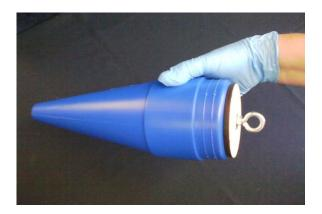
Step 8 - Screw the nut all the way onto the screw eye an insert the screw eye through the flat washer.
