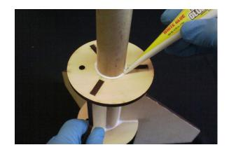
Step 2 – Apply a glue fillet to the inside of each fin where it contacts both the centering rings and the motor tube.
