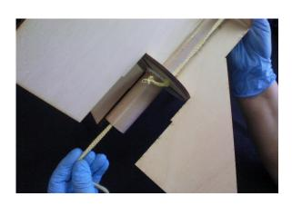
Step 6 - Push the fin can assembly all the way into the crayon tube until the fins stop at the fin slots.
