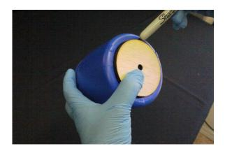
Step 3 - The tail cone bottom surface is now opened to clear the motor installation.
