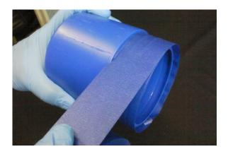
Step 15 - Test that the fit is tight so that the tail cone does not separate during flight.
