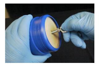
Step 9 - Insert the screw eye assembly into the next largest and then the smaller bulk head last.
