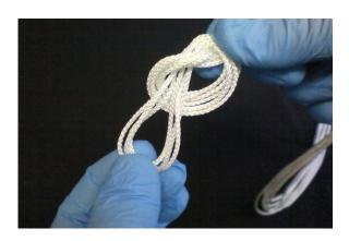
Step 2 - Align the ends of the Kevlar and elastic shock cords and tie a single overhand knot.
