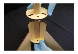
Step 2 - Insert the motor tube into a centering ring until the mark is at the edge of the centering ring.
