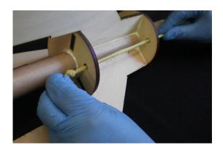
Step 4 - Pull the shock cord through the bottom of the motor tube.
