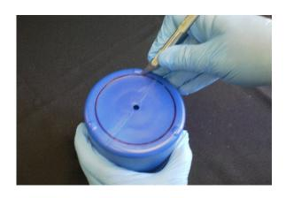
Step 4 - Place the largest bulkhead on top of the smaller bulkheads and insert the t-nut into the center.
