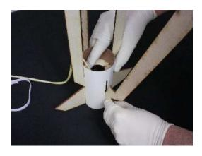
**Step 5 - Insert the motor tube until flush with the table surface.**
