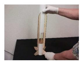
Step 4 Push the two assemblies together over the coupler with the tick marks on both tubes aligned.
