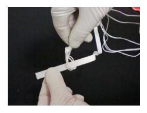
Step 4 - Tie the shock cord to the nose cone with a double knot.
