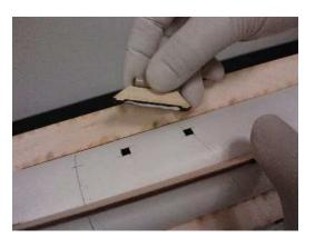
Step 5 - Attach the forward launch lug and stand off pair to the main tube at the forward launch lug slots.
