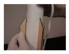
Step 6 - Wrap masking tape around all 4 fins to hold the fins firmly into the slots and against the main tube.
