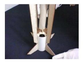
Step 6 - Apply a bead of glue around the centering ring where it contacts both the motor tube and the fin can tube.
