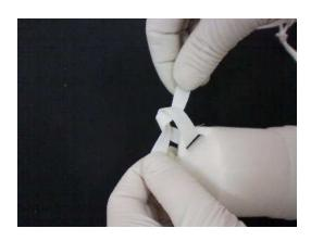
Step 5 - Fold the parachute and roll the shroud lines around the folded parachute.
