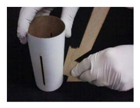
Step 2 – Insert the forward centering ring with the shock cord knot facind down in the tube.
