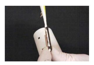
Step 4 - Attach the aft launch lug and stand off pair to the main tube at the aft launch lug slots.
