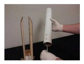
Step 2 Apply a bead of glue around the inside aft end about 1/2" from the aft end.
