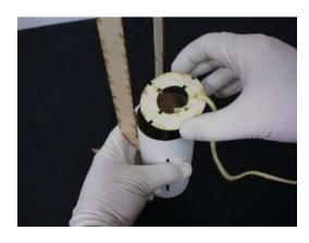
Step 3 - Adjust and lock the centering ring to the fins and hold in place.
