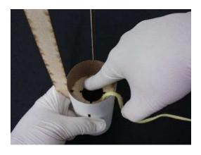
Step 4 - Lift the corners of the centering ring to allow the last two fins to be inserted and lock all fins and the centering ring into place.
