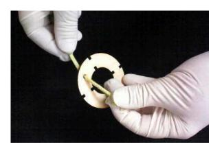
Step 4 - Tie a single knot in the end of the Kevlar shock cord.
