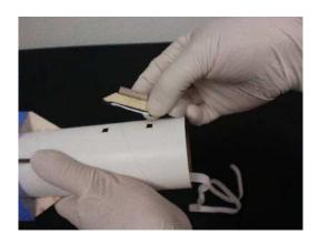
Step 6 - Sight down the launch lug slots to check alignment and adjust if necessary.
