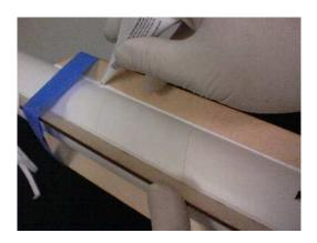
Step 2 - Smooth out the glue at each fillet with a clean finger. Do this for both sides of each fin.
