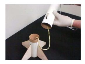
Step 2 Apply a bead of glue around the inside aft end about 1/2" from the aft end.
