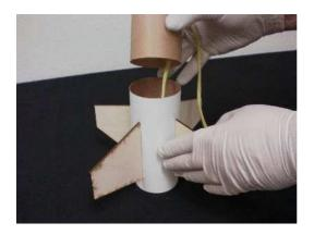
Step 8 - Push the coupler all the way in until it contacts the centering ring and the bead of glue. This will keep the fins and centering ring locked in.
