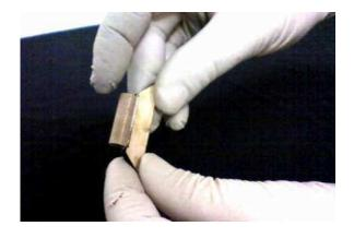
**Step 3 - Apply glue to the longer** bottom of each standoff.
