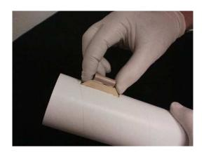
Step 6 - Sight down the launch lug slots to check alignment and adjust if necessary.
