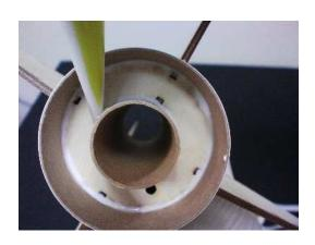
Step 10 - Check that all fins and centering rings both forward and aft are locked in to each other.
