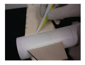
Step 6 - Smooth out the glue at each fillet with a clean finger. Do this for both sides of each fin.
