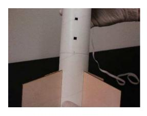
Step 5 - Apply a bead of glue along the length of fins where they intersect the main tube and fin can tubes. Do this for both sides of each fin.
