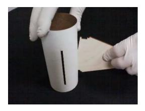
Step 2 – Insert the forward centering ring with the shock cord knot facing down in the tube.
