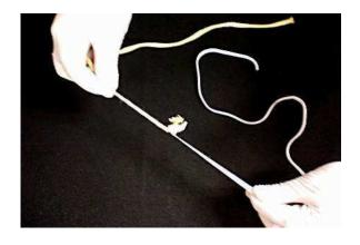
Step 3 - Pull the Kevlar cord through the hole in one centering ring.
