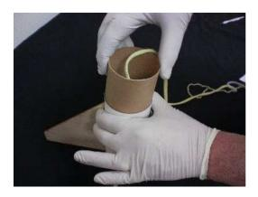
Step 8 - Push the coupler all the way in until it contacts the centering ring and the bead of glue. This will keep the fins and centering ring locked in.
