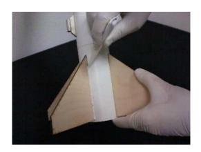
Step 6 - Smooth out the glue at each fillet with a clean finger. Do this for both sides of each fin.
