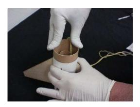
Step 9 - Turn over the fin can and insert the aft centering ring and lock in place with the fins.
