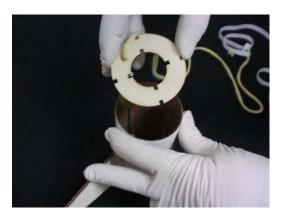
Step 10 - Apply a bead of glue where the aft centering ring contacts the motor tube and inside of the fin can tube.
