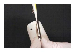
Step 4 - Attach the launch lug and stand off pair to the main tube at the launch lug slots.
