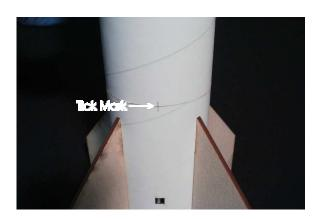
Step 2 - Take the main tube with the launch mount at the top end and insert the shock cord through the end marked with tick mark at the bottom of the tube.
