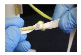
Step 4 - Pull the parachute lines straight to the end and tie a single knot in the end of the parachute lines.
