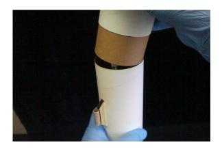
Step 11 – Smooth the glue beads into a fillet using a clean finger. Set aside to dry.
