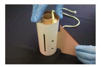
Step 3 - Apply a glue fillet between the inside of the fin can tube and the top centering ring. Take care to not apply glue to the shock cord hole.
