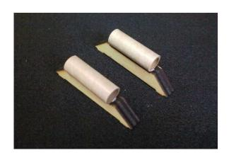
Step 6 - Insert the tabs on the bottom of the lug assembly into the alignment holes on the main tube section.
