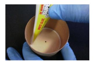
Step 4 - Apply a bead of glue about 1/2" from one end of the payload tube.
