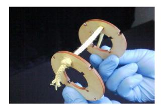
Step 5 - Insert the motor tube and rings w/shock cord knot down into the fin can tube with tick mark on at the top. The tick mark is used to align the tubes.
