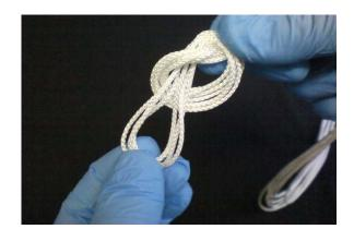
Step 6 - Tie the elastic shock cord to the screw eye on the payload section with a double knot.
