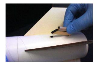
Step 8 - Apply glue to the bottom of the second launch lug assembly.
