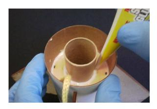
Step 6 - Push the coupler all the way down into the glue fillet on the top centering ring. Set aside to dry.
