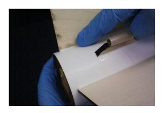
Step 8 - Insert the parachute and shock cords in the top end of the main body tube.
