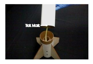
Step 4 - Insert the fin can and coupler into the bottom end of the main tube with the tick mark at the bottom.
