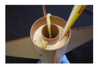
Step 8 - Pull the shock cord all the way through the bottom of the motor tube.
