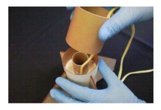
Step 2 - Push in and lock the top centering ring with the top of all 4 fins.
