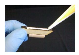
Step 10 - Press the lug assembly firmly onto the fin can section and check both launch lug assemblies to make sure they are aligned with each other.
