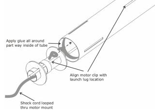
**Step 4** – Pull the shock cord back thru the body tube and out the top of the body tube. Apply a glue fillet at the centering ring and body tube attachment joint. Set aside to dry with the motor mount side of the airframe tube facing up.
