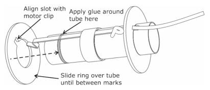
**Step 6** – Apply glue around the inside of the top end of the motor tube and push the thrust ring in until against the motor hook and flush with the end of the motor tube. Set aside to dry thoroughly.
