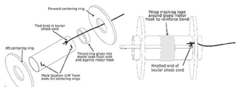
**Step 4** – Glue the thrust ring in the end forward end so that it is against the motor hook and flush with the end of the motor tube.
