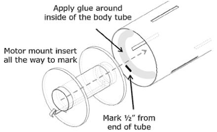
**Step 3** – Apply a glue fillet at the centering ring and body tube attachment joint. Set aside to dry with the motor mount side of the airframe tube facing up.
