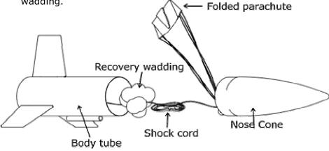
**Step 4** – Fold the parachute 4 times and roll the parachute lines over the folded parachute, insert into the rocket body tube, then insert the nose cone to complete the recovery assembly.
