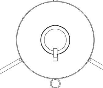
**Step 4** – After the fins and launch lug have dried, apply a thin layer of glue between the body tube and the fins, and the body tube and launch lug with your finger to create a fillet that will strengthen the fins and launch lugs. Set aside to dry. Check the fin alignment to make sure they are 120 degrees apart while drying. Use the fin marking guide to check alignment.
