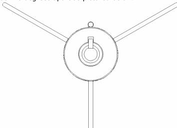
**Step 4** — After the fins and launch lug have dried, apply a thin layer of glue between the body tube and the fins, and the body tube and both launch lug with your finger to create a fillet that will strengthen the fins and launch lugs. Set aside to dry.
