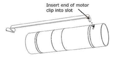
**Step 2** — While holding the motor hook in the slot, apply glue around the motor tube between the wide marks. Push the motor sleeve over the motor hook until the ring is between the wide marks on the motor tube.
